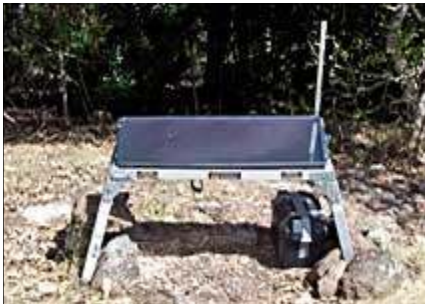
The solar panel has a microphone extension attached at right, a battery on the ground. A phone is tucked under in waterproof casing.
